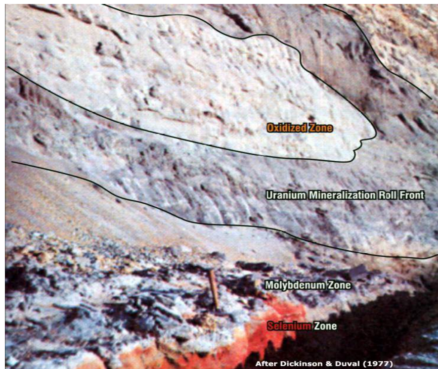
Figure 21 – Typical Roll-Front Uranium Mineralization in an Open-Pit Mine of the 1970s in South Texas (Campbell, et al. , 2004)
