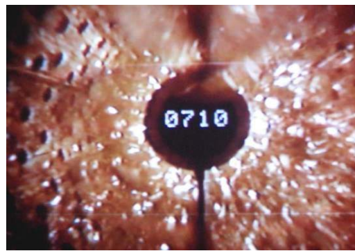
Figure 29 – Natural Gas Bubbles at 710 Feet Entering the Well at the Top Screened Zone (From Campbell and Wise, 2013)
